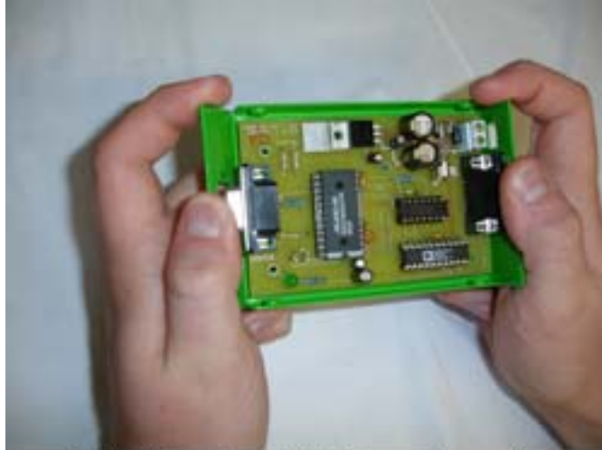
Using force to stretch the u-shape to fit the PCB
